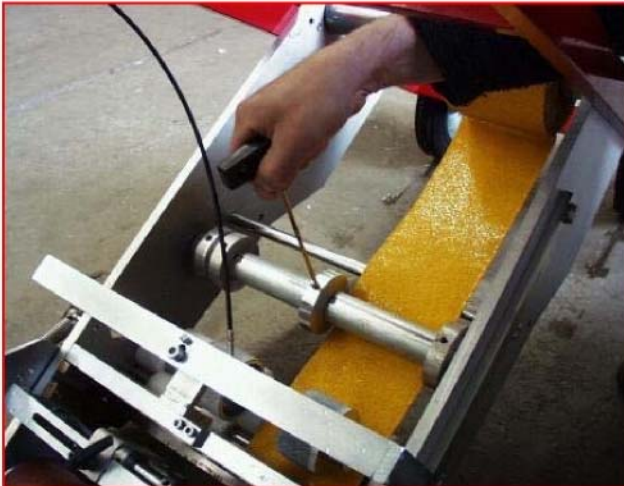
Figure 4: Adjustment of the upper tape guide rolls
