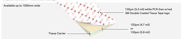
These acrylic multipurpose tapes are available in 120-micron (56212) and 150-micron (56215) thicknesses and come on a PCK liner. The tissue carrier provides dimensional stability and improved handling for easier die-cutting and laminating.
